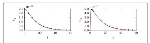
**Fig. 8** Migration of a floating rigid circular disk to the center line of a channel: vertical position  $r_y$  and horizontal velocity  $u_x$  of the center of the floating circular disk in the channel computed with the proposed formulation and an initial particle spacing of  $\Delta x = 2.0 \times 10^{-4}$  (red dashed line) and  $\Delta x = 1.0 \times 10^{-4}$  (black solid line) compared to the reference solution [8] (crosses)
