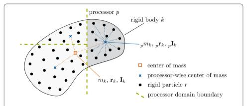
**Fig. 4** Parallel distribution of a rigid body k with rigid particles r over several processors p illustrating the evaluation of mass  $m_k$ , center of mass position  $\mathbf{r}_k$ , and mass moment of inertia  $\mathbf{I}_k$  via processor-wise mass  $p_k$ , center of mass position  $p_k$ , and mass moment of inertia  $p_k$
