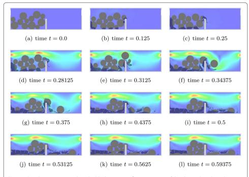
**Fig. 13** Powder grains exposed to a highly dynamic gas flow: time series of the obtained results with magnitude of the velocity field ranging from 0.0 (blue) to 600.0 (red)
