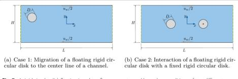
Fig. 7 A rigid circular disk floating in a shear flow: geometry and boundary conditions of two different cases
