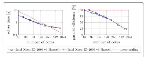
**Fig. 18** Strong scaling analysis of parallel computational framework: solver time per time step (left) and parallel efficiency given in percent of linear scaling (right) for a three-dimensional problem consisting of approximately  $3.79 \times 10^6$  particles on up to 768 cores
