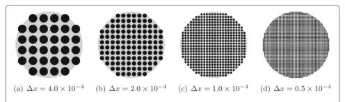
**Fig. 6** Spatial discretization of a rigid circular disk: resulting spatial discretization of a rigid circular disk with rigid particles for selected values of the initial particle spacing  $\Delta x$
