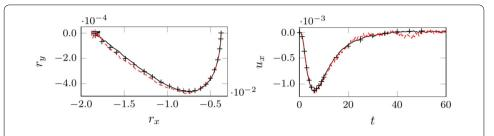
**Fig. 9** Interaction of a floating rigid circular disk with a fixed rigid circular disk: trajectory and horizontal velocity  $u_x$  of the center of the floating circular disk in the channel computed with the proposed formulation and an initial particle spacing of  $\Delta x = 2.0 \times 10^{-4}$  (red dashed line) and  $\Delta x = 1.0 \times 10^{-4}$  (black solid line) compared to the reference solution [8] (crosses)
