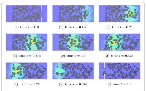
**Fig. 15** Gastric disintegration of food boluses: time series of the obtained results with magnitude of the velocity field ranging from 0.0 (blue) to 120.0 (red)
