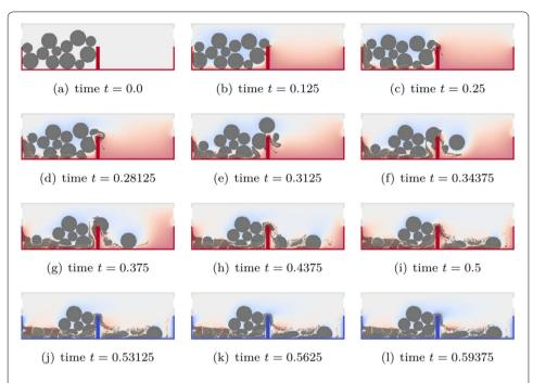
**Fig. 12** Powder grains exposed to a highly dynamic gas flow: time series of the obtained results with temperature field ranging from 0.0 (blue) to 100.0 (red)
