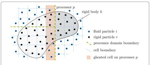
**Fig. 2** A fluid–solid interaction problem consisting of a rigid body k with affiliated rigid particles r and surrounding fluid particles i distributed over several processors p according to a spatial decomposition approach
