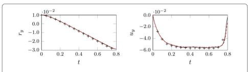
**Fig. 11** A rigid circular disk falling in a fluid column: vertical position  $r_y$  and vertical velocity  $u_y$  of the center of the circular disk in the fluid column computed with the proposed formulation and an initial particle spacing of  $\Delta x = 2.0 \times 10^{-4}$  (red dashed line) and  $\Delta x = 1.0 \times 10^{-4}$  (black solid line) compared to the reference solution [8] (crosses)
