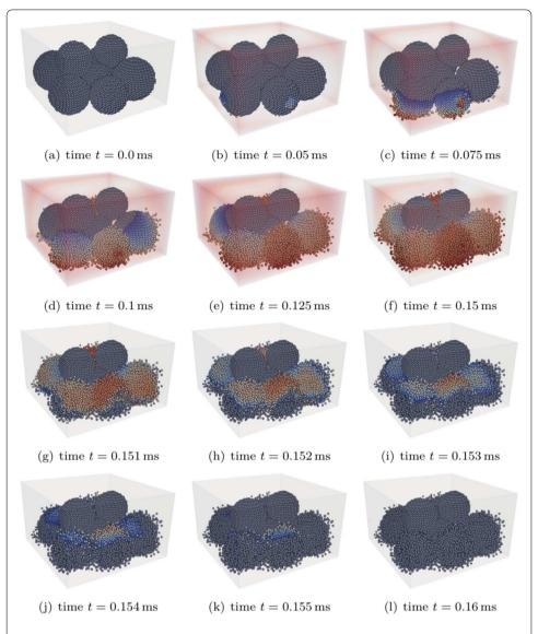
**Fig. 14** Three-dimensional powder melting setup with representative material parameters: time series of the obtained results with temperature field ranging from 1700 K (blue) to 1800 K (red)
