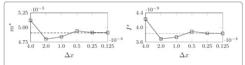
**Fig. 5** Spatial discretization of a rigid circular disk: mass  $m^5$  and mass moment of inertia  $l^5$  of a rigid circular disk for different values of the initial particle spacing  $\Delta x$  (solid line) compared to the analytical solution (dashed line)
