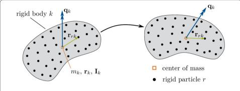
**Fig. 3** Orientation of a rigid body k with rigid particles r and their relative position  $\mathbf{r}_{rk}$  described via a unit quaternion  $\mathbf{q}_k$  at different times
