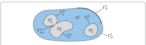
**Fig. 1** Domain  $\Omega$  consisting of several disjunct domains, the fluid domain  $\Omega^f$  and the solid sub-domains  $\Omega^{\Sigma}$ representing rigid bodies k, with fluid-solid interface  $\Gamma_k^{f_5}$  and solid-solid interface  $\Gamma_{kl}^{55}$  in the event of contact between the rigid bodies k and  $\hat{k}$
