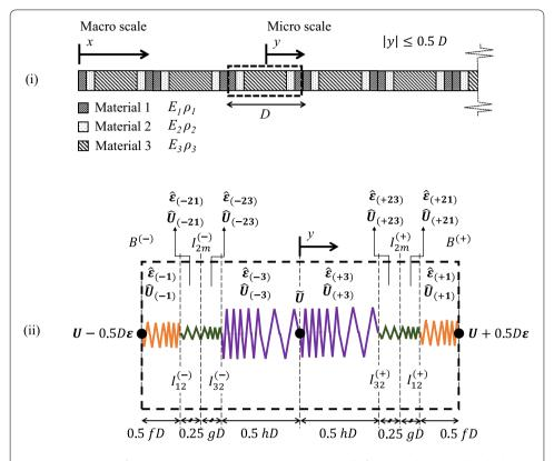
**Fig. 4** i Schematics of a periodic layered composite bar with a unit cell of size *D.* ii The unit cell is idealised as a series of springs over eight segments. The mass of each constituent material is evenly distributed across the corresponding segment within the unit cell
