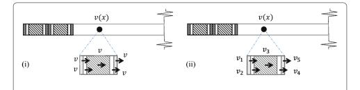
**Fig. 1** Possible transient responses within a unit cell when a macro point x is subjected to velocity v(x): **i** the entire unit cell moves with the same velocity; **ii** the stiff layer, compliant layers and matrix material move at different velocities
