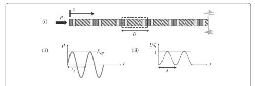
**Fig. 5 i** Schematics of a periodic layered composite bar with underlying unit cell of size D, subjected to a sinusoidal load P at x = 0. **ii** Sinusoidal load P with amplitude  $E_{eff}$  over two periods,  $2t_d$ . **iii** Normalised non-dispersive displacement response predicted by a standard elastic effective medium
