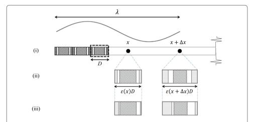
**Fig. 2** i Two length scale parameters  $(\lambda, D)$  characterising the problem. ii When  $O(\lambda) \gg O(D)$ , a unit cell at each macro point x deforms locally to satisfy the imposed macro strain. iii When  $O(\lambda) \to O(D)$ , the deformation within each unit cell is furthermore influenced by the short range forces from neighbouring cells
