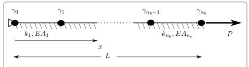
**Fig. 1** Linear elastic straight bar on an elastic support, with  $n_b$  sections. The bar is fixed at the start and has a concentrated load at the end
