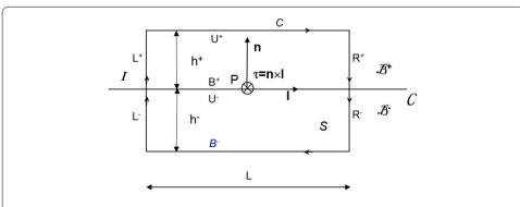
**Fig. 1** Burgers circuit  $C = U^+ \cup R^+ \cup R^- \cup B^- \cup L^- \cup L^+$  across an interface I separating the body  $\mathcal B$  into domains  $\mathcal B^-$ ,  $\mathcal B^+$ . 1 is the unit tangent to curve  $\mathcal C$ ,  $\mathbf n$  is the unit normal to interface I, and  $\mathbf \tau = \mathbf n \times \mathbf 1$  the "tangent normal" to the bounded surface I and curve I0.
