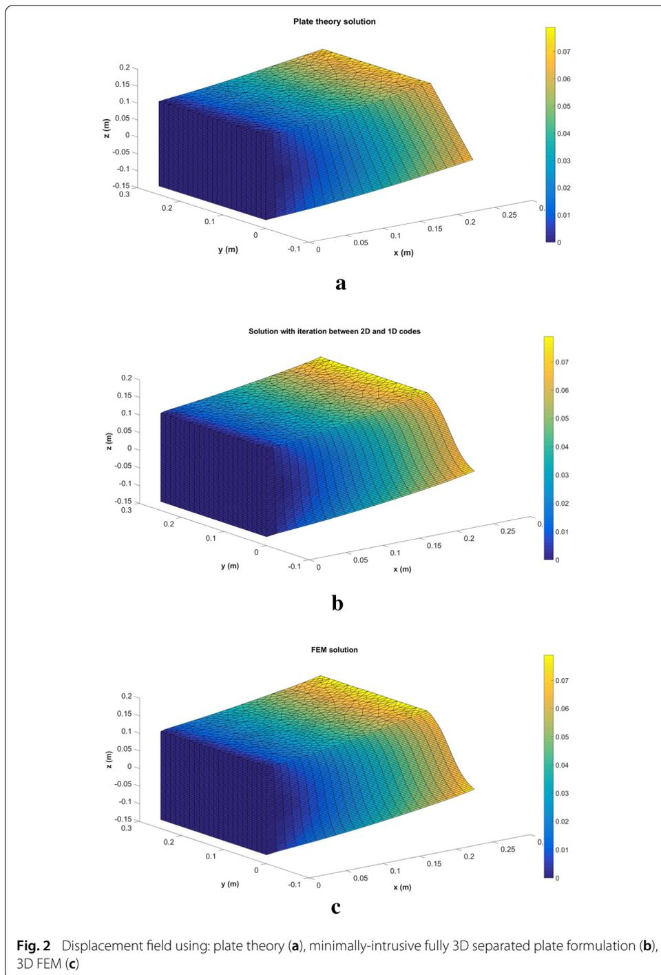
**Fig. 2** Displacement field using: plate theory (a), minimally-intrusive fully 3D separated plate formulation (b), 3D FEM (c)
