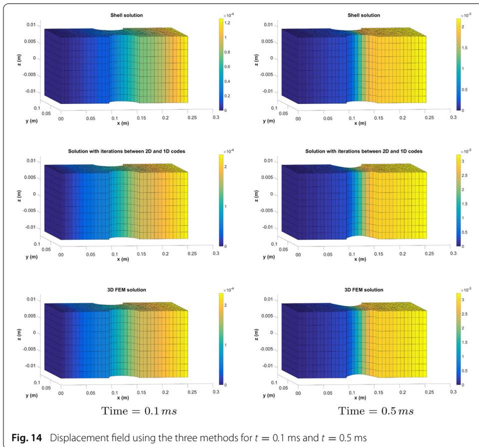
**Fig. 14** Displacement field using the three methods for  $t = 0.1 \text{ ms}$  and  $t = 0.5 \text{ ms}$
