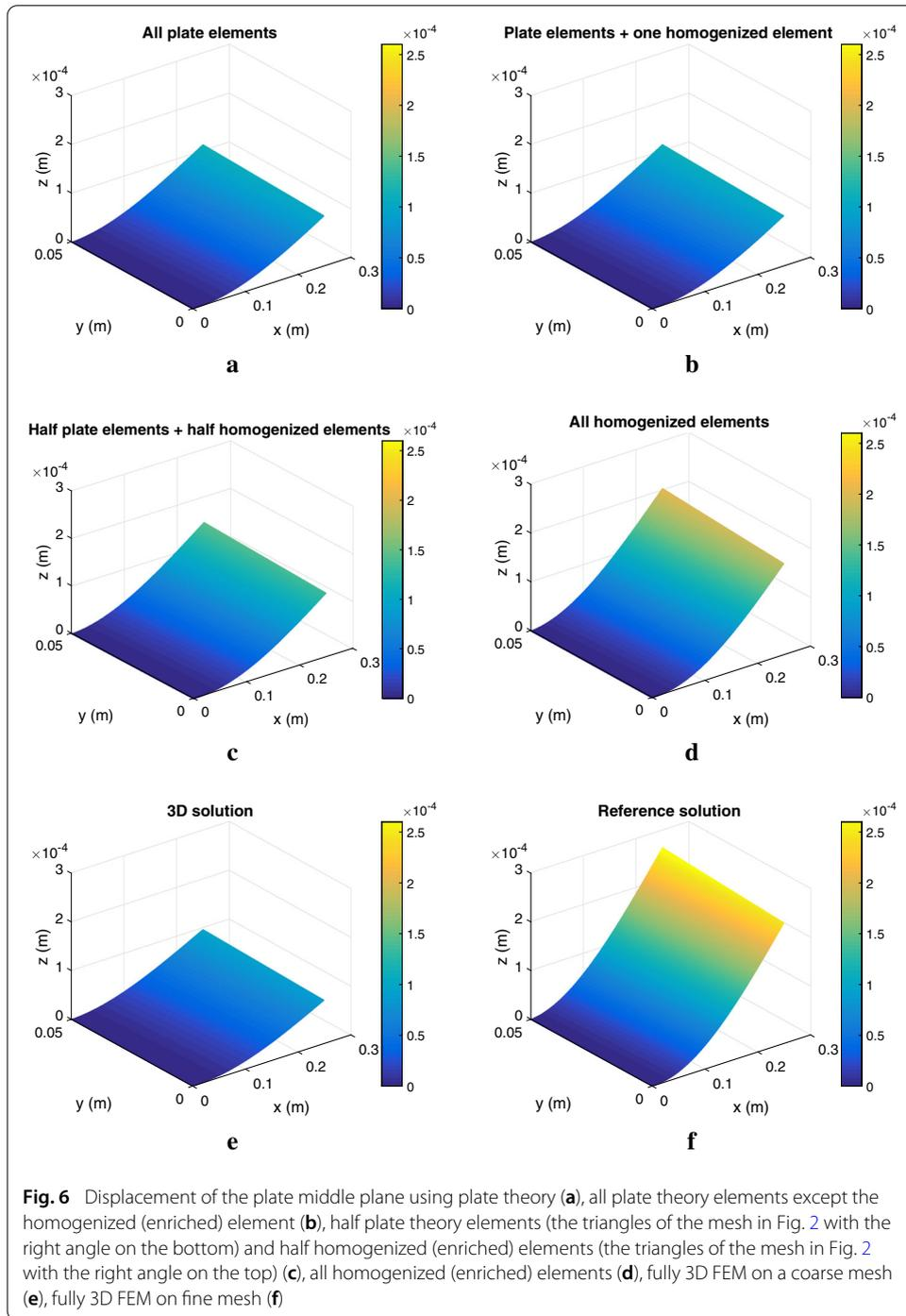
It is important to note that even when all the element are enriched, the solution exhibits a gap with respect to the reference solution. This gap can be explained by the fact that despite of the valuable enrichments introduced at the elements level, at the elements boundaries standard plate kinematics is enforced with its consequent impact on the resulting kinematic that continue to be too constrained with respect to a fully 3D kinematics.
