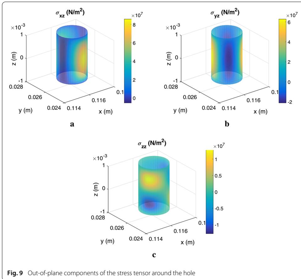
**Fig. 9** Out-of-plane components of the stress tensor around the hole
