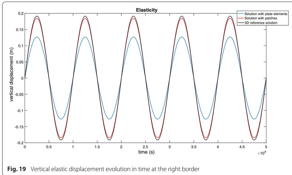
**Fig. 19** Vertical elastic displacement evolution in time at the right border
