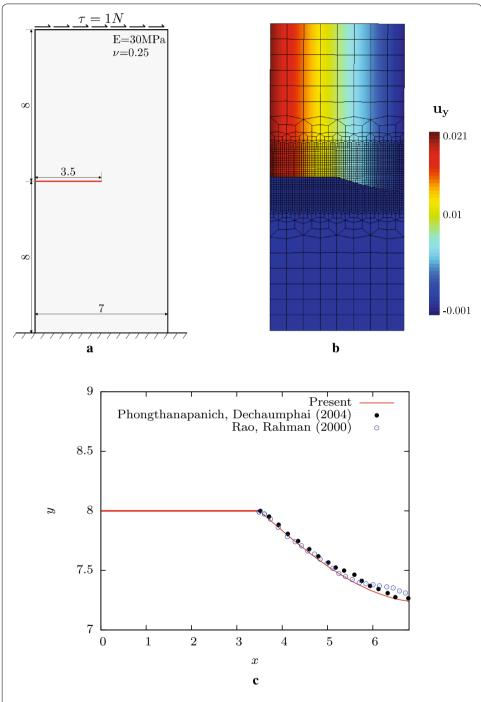
**Fig. 8** Single edge crack plate under mixed mode loading: **a** Geometry, material parameters and loading conditions; all dimensions are in mm. **b** Contours of displacement in vertical direction. **c** Crack tip trajectory
