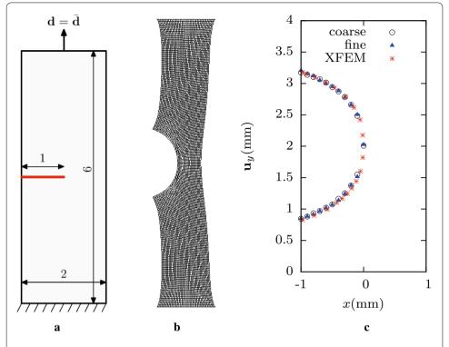
**Fig. 6** Crack tip blunting. **a** Geometry. All dimensions are in mm. **b** Deformed configuration. **c** Plot of vertical displacement of crack surface nodes against their horizontal position in reference state. XFEM results for comparison are taken from [30]
