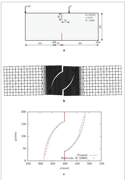
**Fig. 10** Four point bending beam with two notches: **a** Geometry, material parameters and loading conditions (not to scale). All dimensions are in mm, **b** crack path, **c** comparison of crack tip trajectories
