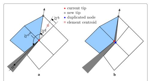
**Fig. 5** Nodal release technique **a** splitting an element to allow crack propagation along diagonal, **b** modify connectivity locally near crack tip; the crack opening is shown only for visualization
