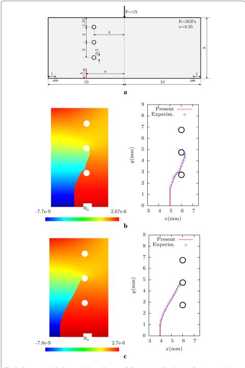
Fig. 9 Bittencourt's drilled plate problem. **a** Geometry, **b** Simulation-1, **c** Simulation-2. Experimental values for comparison are taken from [7]
