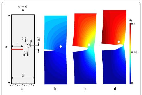
**Fig. 12** Plate with a hole. **a** Geometry (not to scale). All dimensions are in mm. **b** The configuration at which the crack starts propagating. **c** An intermediate configuration. **d** Final configuration
