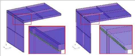
Figure 4 Conforming (left) and mortar discretizations (right) of the structure whose geometry is described in Figure 2. The thin elastomer layer is condensed into the mortar interface.
