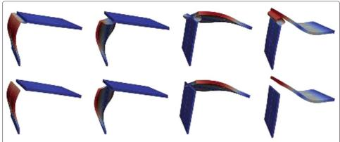
**Figure 6 Comparison between eigenmodes 1, 3, 4, 7.** Top row: conforming, hexahedral discretization. Bottom row: new mortar method. Note that the greyscale shows the displacement.
