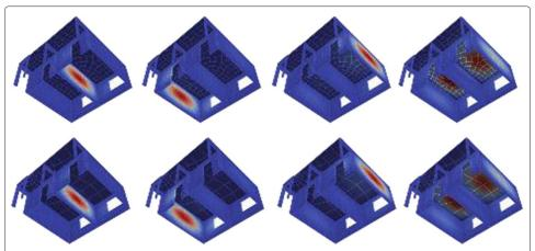
**Figure 11 Comparison between eigenmodes 1, 2, 3, 4.** Top row: resulting from the conforming discretization corresponding to Figure 8, Bottom row: non-conforming discretization corresponding to Figure 10.
