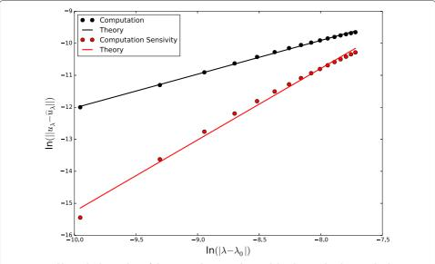
**Figure 2 Red line:** The logarithm of the error relative to the model reduction by the enriched POD basis. Black line: The logarithm of the error relative to the model reduction by the reference POD basis.
