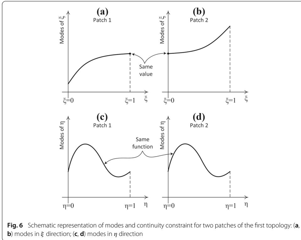
**Fig. 6** Schematic representation of modes and continuity constraint for two patches of the first topology: **(a, b)** modes in  $\xi$  direction; **(c, d)** modes in  $\eta$  direction
