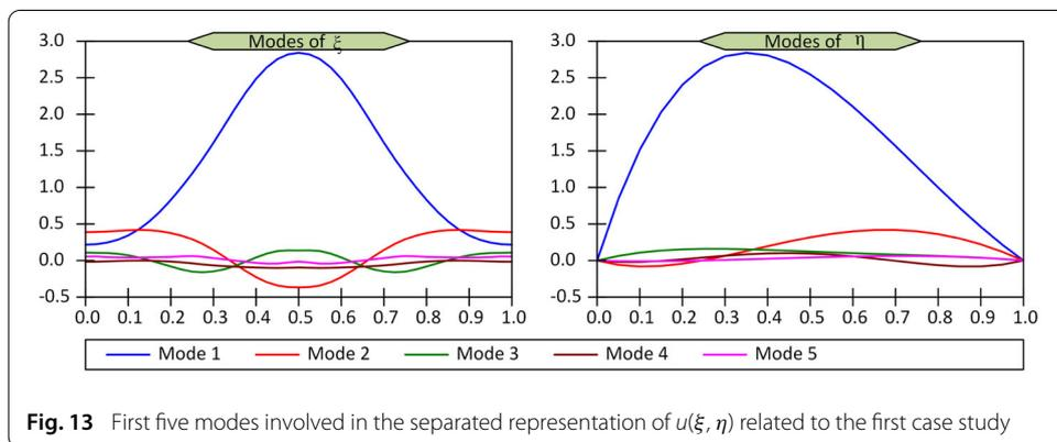
The first five modes involved in the separated representation of  $u(\xi, \eta)$  are shown in Fig. 13. The contours of the reconstructed field in the physical and computational domains are shown in Fig. 14. The computed PGD solution is compared with exact one in Fig. 15 along the line  $x = 0$  for  $1 < y < 4$ , proving the excellent accuracy of the computed solution.
