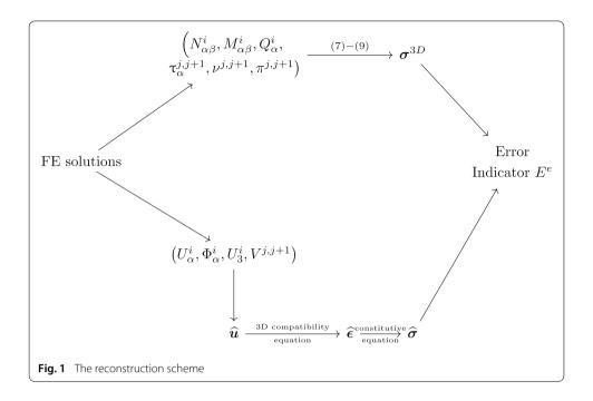
$u_{\alpha}^{d}$  is piecewise-linear and complies with Eqs. (15), (16) but is not continuous at the interfaces. To achieve our initial goal,  $\widehat{u}_{\alpha}$  is obtained by performing an L2-projection of  $u_{\alpha}^{d}$  over piecewise linear continuous functions over z.
