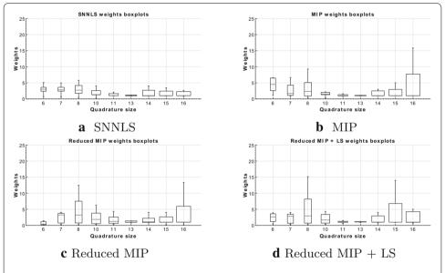
**Fig. 16** Hyper-reduction weights boxplots for constraints reduction formulations in comparison with the SNNLS and MIP methods
