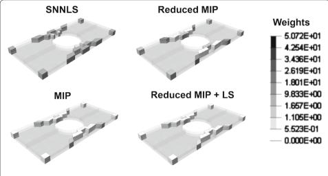
**Fig. 13** Element selection for the hyper-reduced integration schemes of size seven computed with the different methods
