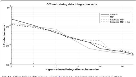
**Fig. 11** Offline training data relative L2 error (33) of SNNLS and proposed hyper-reduced methods. Hyper-reduced integration schemes sizes range from 6 to 17
