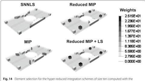
Fig. 14 Element selection for the hyper-reduced integration schemes of size ten computed with the different methods
