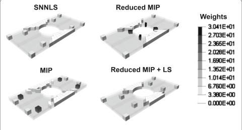
**Fig. 15** Element selection for the hyper-reduced integration schemes of size fourteen computed with the different methods
