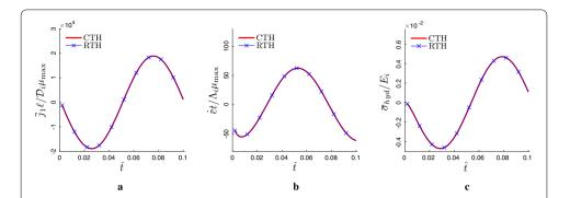
**Fig. 6** Comparison between the macroscopic quantities computed with the conventional computational homogenization (based on the fully resolved microscale RVE analysis), shown in red, and the reduced order homogenization, shown in blue. **a** Macroscopic mass flux  $j_1$  in  $\mathbf{x}_1$  direction, **b** macroscopic concentration rate  $\dot{c}$  and **c** macroscopic hydrostatic stress  $\bar{\sigma}_{hyd} = \frac{\bar{\sigma}_{11} + \bar{\sigma}_{22}}{3}$
