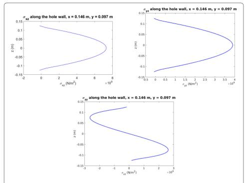
**Fig. 7** Out-of-plane stress tensor components around the hole for x = 146 mm and y = 97 mm using the minimally-intrusive fully 3D separated plate formulation
