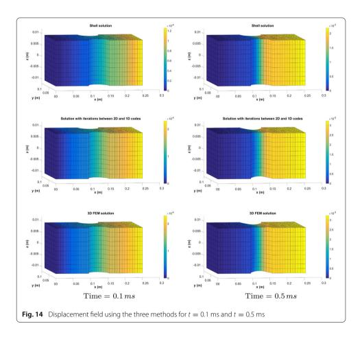
[9]. The problem is solved in the time interval [0, 50] ms with a time step  $\Delta t = 10^{-4}$  ms which ensures the stability of the explicit method. In order to get the stationary solution the traction is applied gradually as depicted in Fig. 13 and a Rayleigh damping (proportional to the mass) is used. Figs. 14, 15 and 16 compares the solution obtained with the three methods at different times. For this problem the 2D solution is given by shell theory [1] as
