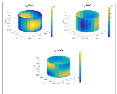
**Fig. 5** Out-of-plane stress tensor components around the hole using the minimally-intrusive fully 3D separated plate formulation
