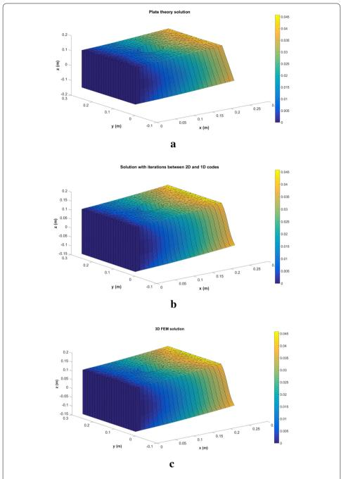
**Fig. 4** Displacement field using: plate theory (**a**), minimally-intrusive fully 3D separated plate formulation (**b**), 3D FEM (**c**)
