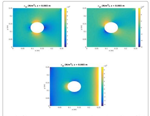
**Fig. 6** Out-of-plane stress tensor components in the  $z=65\,\mathrm{mm}$  plane using the minimally-intrusive fully 3D separated plate formulation
