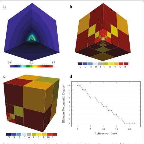
**Fig. 7** Singular cube: solution and discretization. **a** Numerical solution gradient magnitude. **b** Ansatz order close to singular corner. **c** Ansatz order on side. **d** Polynomial degree distribution on the line x = 0, y = 0
