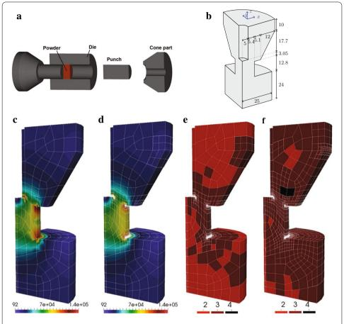
**Fig. 11** Geometrically complex example: problem description, solution and discretization. **a** Schematic sketch of the FAST process from [49]. **b** Geometry description in [mm]. **c** Solution gradient magnitude on initial mesh. **d** Solution gradient magnitude on refined mesh. **e** Ansatz order after 30 steps. **f** Ansatz order after 57 steps
