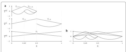
**Fig. 1** Example of one-dimensional multi-level mesh and basis functions. **a** Multi-level mesh. **b** Basis functions for analysis
