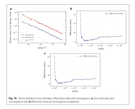
performed. In the asymptotic part, the grid is fixed and just p-refinements are employed. Here, a clear exponential behavior is shown.
