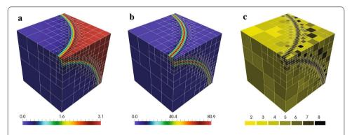
**Fig. 9** Shock problem: solution and discretization. **a** Numerical solution. **b** Numerical gradient magnitude. **c** Ansatz order
