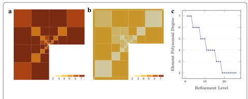
**Fig. 5** L-shape domain: discretization. **a** Ansatz order. **b** Ansatz order around singular corner. **c** Polynomial degree distribution on the line  $x \ge 0$ , y = 0
