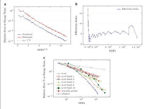
**Fig. 8** Singular cube: error estimates, effectivity index and convergence. **a** Error estimates and convergence rate. **b** Effectivity index. **c** Convergence comparison
