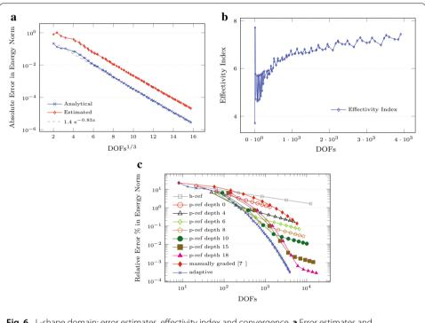
**Fig. 6** L-shape domain: error estimates, effectivity index and convergence. **a** Error estimates and convergence rate. **b** Effectivity Index. **c** Convergence comparison
