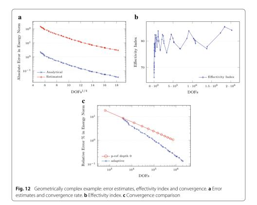
the error and the adaptive procedure drastically improves the convergence rate of the standard p-extension, as clearly shown in Fig. 12a-c.
