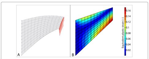
Figure 8 Cook's membrane obtained after iteration nine: (A) undeformed configuration with applied forces (red) and boundary conditions (blue), (B) deformed configuration with equivalent plastic strain (-).
