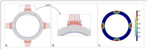
Figure 11 Circular, flat plate after iteration five: (A) undeformed configuration with applied forces (red) and boundary conditions (blue), (B) zoom, (C) deformed configuration with equivalent plastic strain (-).
