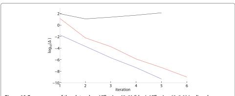
Figure 10 Convergence of the plate when  $\{E^p,\alpha\}=\{0,0\}$  (blue),  $\{E^p,\alpha\}=\{0,0.1\}$  (red) and  $\{E^p,\alpha\}=\{-0.1,0\}$  (black).
