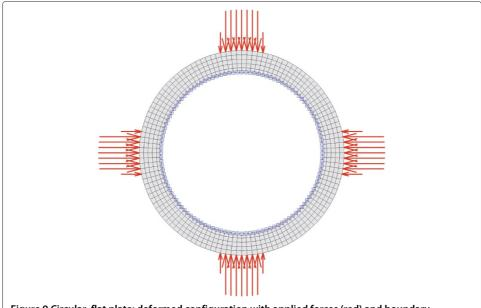
Figure 9 Circular, flat plate: deformed configuration with applied forces (red) and boundary conditions (blue).
