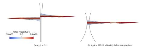
**Fig. 9** Detail study of the resulting line force distributions for two displacement values obtained for the case  $\tilde{f}_{\min, \square} = -1$ . For clarity, the fibers are depicted as their centerlines and forces are shown for the left fiber only. Note that both pictures show details of the entire system and are not to scale
