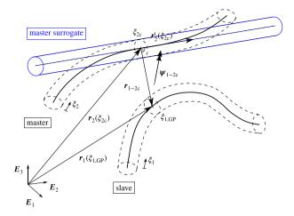
**Fig. 3** Illustration of the section–beam interaction potential (SBIP) approach. The actual, deformed volume of the second interaction partner ("master") is approximated by a surrogate body (blue) located at the closest point  $\xi_{2c}$  to a given integration point  $\xi_{1,GP}$  of the first interaction partner ("slave"). Distance vector  $\mathbf{r}_{1-2c}$  and relative rotation vector  $\mathbf{\psi}_{1-2c}$  uniquely describe the mutual separation and orientation
