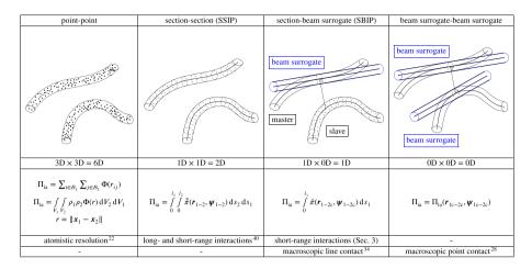
Fig. 6 Classification of formulations for beam-beam interactions
