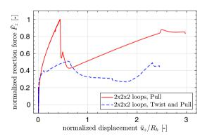
**Fig. 15** Force-displacement curves for the decisive phase, i.e.,  $2 \le t < 5$  in the "Pull" scenario and  $2 \le t < 7$  in the "Twist & Pull" scenario. Force values are normalized with respect to the maximal pull-off force  $F_{Z,\max}$
