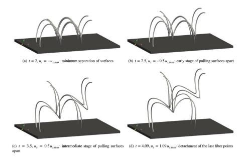
**Fig. 13** Sequence of simulation snapshots of the "Pull" scenario. Top surface is hidden for better visibility of the fibers
