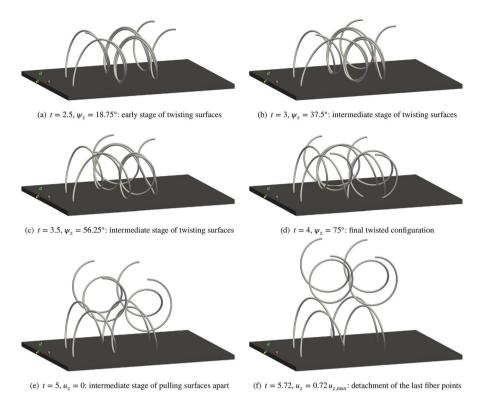
**Fig. 14** Sequence of simulation snapshots of the "Twist & Pull" scenario. Top surface is hidden for better visibility of the fibers. Note that until time t = 2, this scenario is identical to the "Pull" scenario shown in Fig. 13
