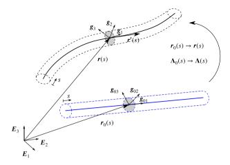
**Fig. 2** Example configurations and kinematics of the Cosserat continuum formulation of a beam to illustrate the field of centroid positions r(s, t) and material triad field  $\Lambda(s, t)$ : Initial, i.e., stress-free (blue) and deformed (black) configuration. Straight configuration in the initial state is chosen here as an example, although the applied beam theory is more general
