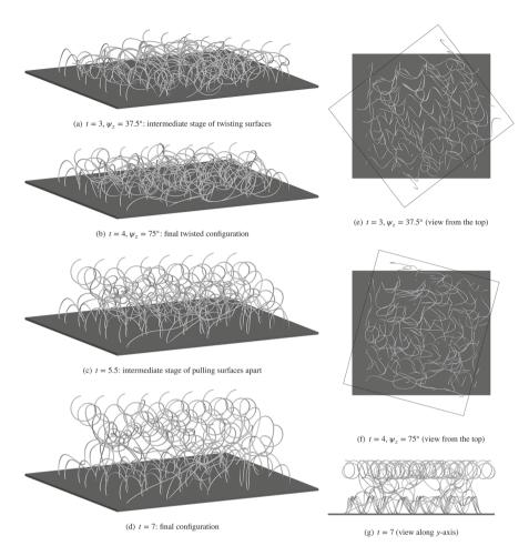
**Fig. 17** Sequence of simulation snapshots of the "Twist & Pull" scenario with  $2 \times 8 \times 8$  loops. Top surface is hidden for better visibility of the fibers (and outlined by the black rectangle in the views from the top)
