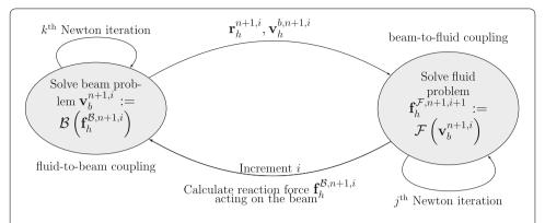
**Fig. 5** Visualization of the one-way fluid and solid coupling schemes. In the visualization,  $\mathcal{B}$ ,  $\mathcal{F}$  represent suitable operators for the solution of the nonlinear beam problem, and for the solution of the nonlinear fluid problem, respectively
