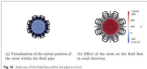
domain. Figure 18a shows the initial position of the stent at the edge of the outer fluid mesh layer.
