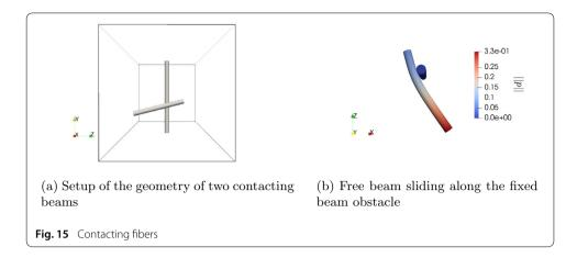
Nevertheless, we will show the suitability of the proposed approach to model fluid-driven beam-to-beam contact under rather small violations of the one-way-coupling assumptions and moderate FBI penalty parameters, using a penalty contact method as introduced in [54].
