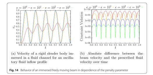
In this example, the fluid is again assumed to be contained in a hexahedron of dimensions  $1 \times 1 \times 3$  as introduced in "Fixed obstacle immersed in a fluid channel". Only now all DoFs in channel direction are set to be free and a velocity of zero is prescribed in both other directions, leading to a pseudo one-dimensional setup. In order to analyze the time-dependent behavior of the beam in dependence on the penalty parameter, an oscillatory inflow velocity
