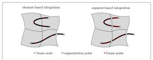
**Fig. 4** Segmentation of the beam element for stable and accurate numerical integration as presented in [24]: circles and crosses denote beam nodes and quadrature points, respectively. The squares subdivide the beam into integration segments, such that an integration cell on the beam does not cross element boundaries of the fluid mesh to not integrate across weak discontinuities
