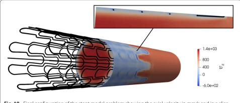
**Fig. 19** Final configuration of the stent model problem showing the axial velocity in mm/s and in a slice through the origin at a 45° angle
